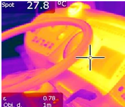
Fig. 7. Temperature measured with thermal image camera on the driver area on the bus
